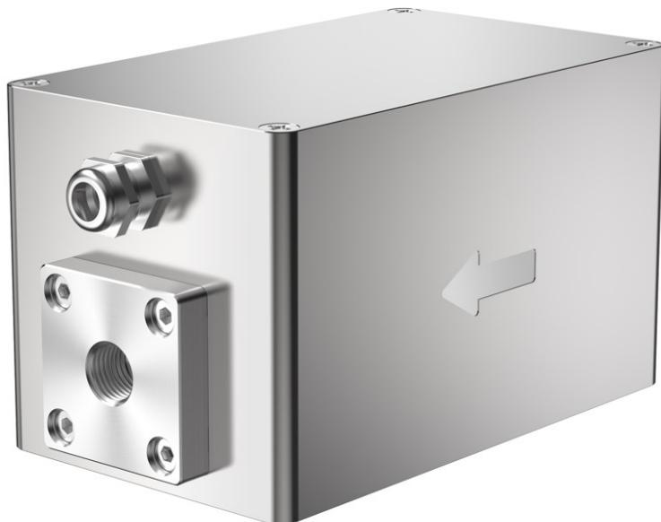
The OMS-300 is equipped with an industry-leading high-precision and high-stability wear debris detection module. This module employs an advanced multi-coil magnetic field disturbance detection principle, combined with a high-performance data sampling and processing unit, to achieve real-time capture and cumulative output of ferromagnetic particles  $\geq 40\mu\text{m}$  and non-ferromagnetic particles  $\geq 150\mu\text{m}$ .
