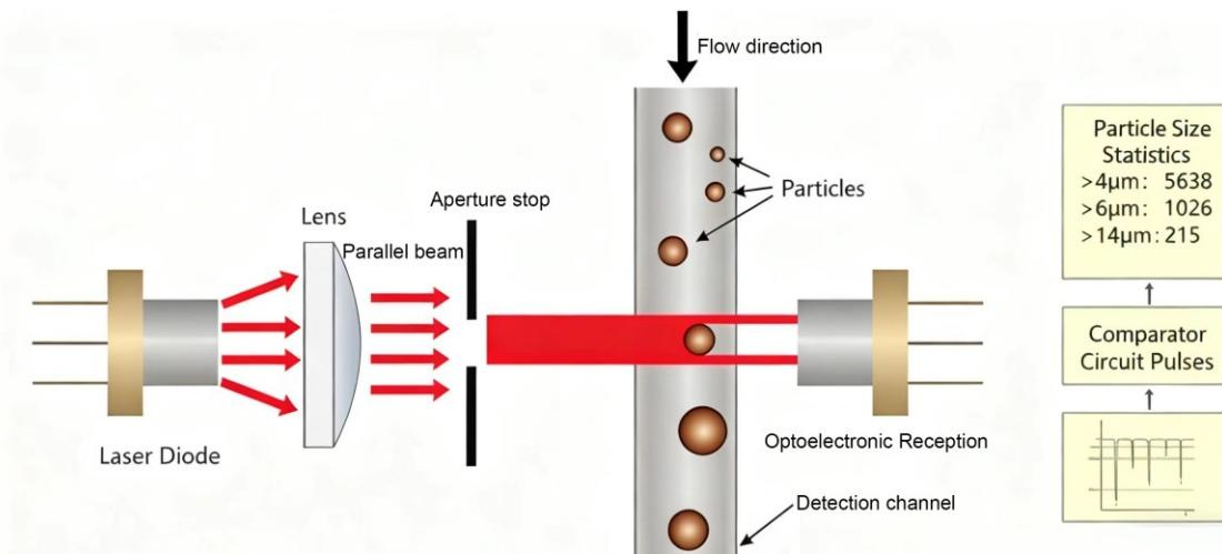
OPC-500 features a high-performance semiconductor laser that, via a collimating lens, directs a parallel beam into the oil detection channel inside the counter. Paired with a high-efficiency PIN photodetector serving as the signal-receiving unit, it enables real-time monitoring of particle count and contamination levels.
